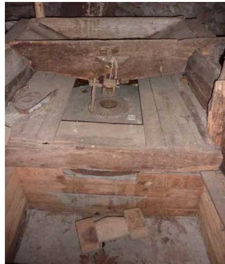
The metallic pressure pipe and the grinding mechanism of one of the two mills we are going to see.
