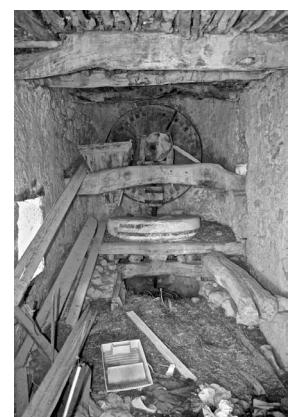
a typical mechanical part of a U-shape floor type windmill in Mirabello
