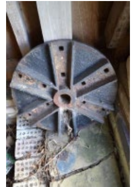
Figs. 6 & 7. Detail on the body, and the sail hub (note the tapered slots for the sails).
