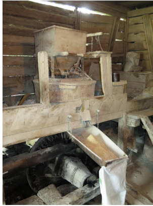
20 Wheelpit, hopper and stones
