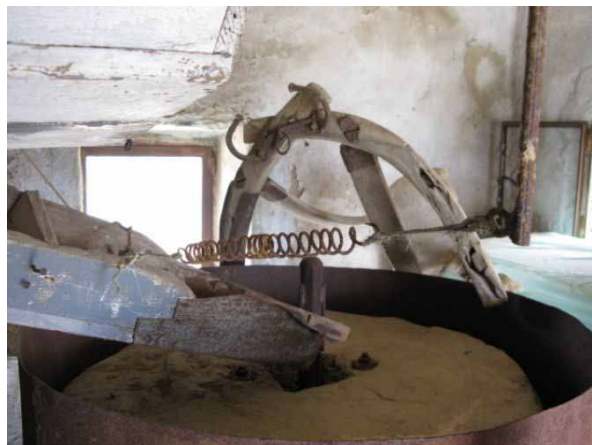
The spring regulating the amount of seeds falling
