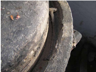
The sesame paste guide towards the lower millstone hole
