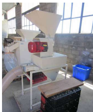
The new Heger spelt-peeler, with the grain cleaner from the same firm behind.
