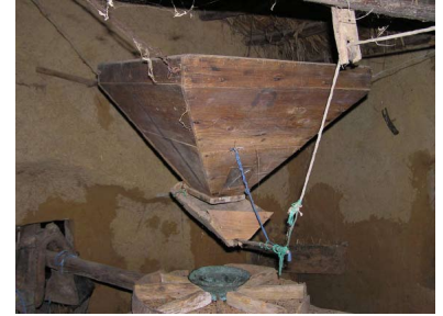
The hopper and the spoke mechanism on the upper millstone to shake down the seed in the millstones
