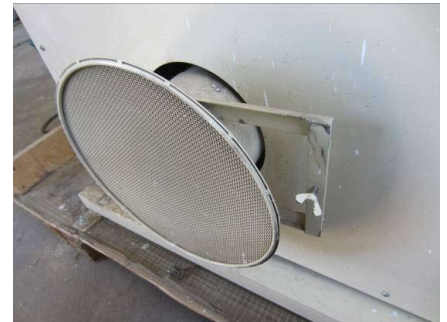
A flat slide to adjust the flow through the fan is missing.
