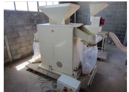
The Heger grain cleaner. Behind the electrical control box, one tilt-adjuster can be seen.
