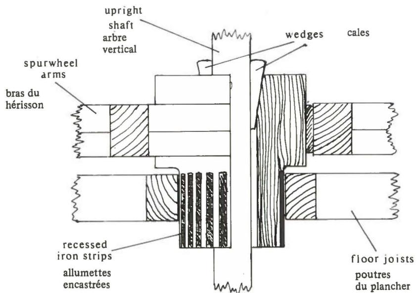
part-section of spurwheel bearing
