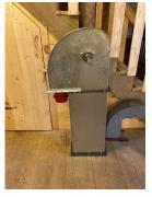
Custom food stainless steel elevator head. Minimum conveyance 110 bushels/hr. The head pictured is for non-organic grain and has a 24'6" discharge height.
