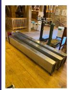
Custom stainless elevator sections for organic stones. 30' discharge height. Slide gate access on every floor level for clean out.
