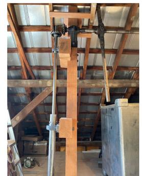
*Vertical shaft extended to 3rd floor and disengagement levee.*
