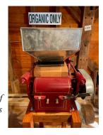
Roller Mill- 12"x6" capacity of 350lbs/hr @ 3hp. 20 corrugations per inch.
