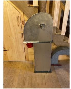
*Custom food grade stainless steel elevator head. Minimum conveyance 110 bushels/hr. The head pictured is for non-organic grain and has a 24'6" discharge height.*
