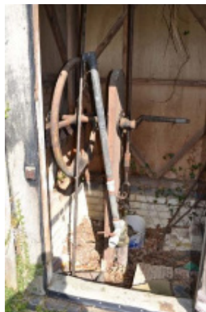
The borehole pump, which can be driven by wind or by hand (both photos May 2016).
