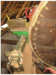
The outside surface was now a series of flats, which had to be machined round, also using the lathe.
