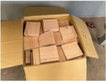
Blocks of Rubberwood or Para wood from a plantation in Malawi, prepared on one side with the required radius to match the brake wheel. The edges were chamfered too. We worked out that
