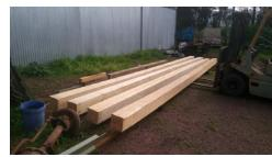
Spruce beams 200mm square and 8m long are in my yard for use as stretchers, braces and tail-pole.
