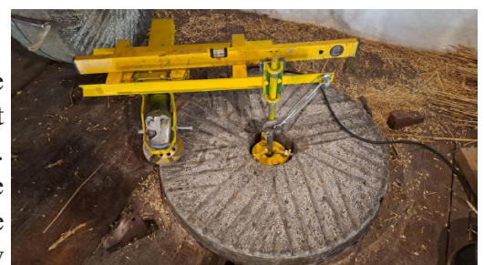
Fig 8. My rotating grinding rig, the carriage with the grinder can be moved inward on the rail.
