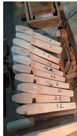
Graded roots of the cogs according to how they fitted in one socket, for selective assembly.
