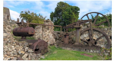
Fig. 19 Steam powered mill with horizontal rollers at estate Annaly
