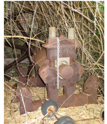
Fig. 22 The steam-powered horizontal mill at Rust op Twist only has one of the three crushing rollers remaining in place
