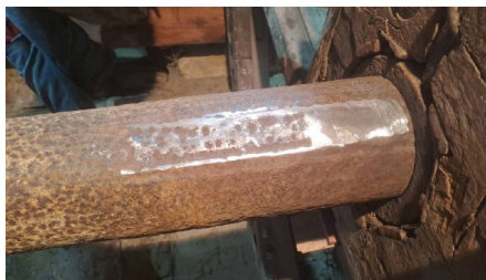
Extending the flat on the shaft, using a grinder, then a flat file.
