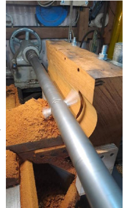
The fly-cutter machining wood away from one half-block.
