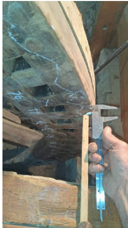
Checking the run-out.
