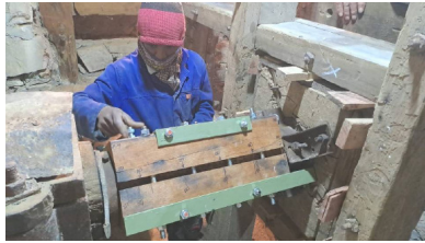
Pierrie assembling the block with the long angles just touching the wooden block in the hub.
