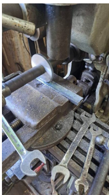
Machining the flat key on the Dainichi. See the head of the shaper below?
