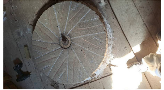
11 harps, laid out for right hand rotation. I was happy with the bedstone.
