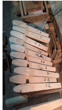
Fitting new cogs to the sockets. I was showing Thys how stiffly they should fit.
