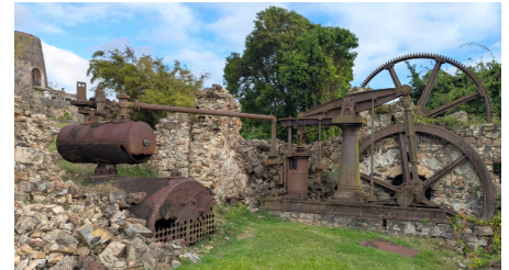
Fig. 19 Steam powered mill with horizontal rollers at estate Annaly
