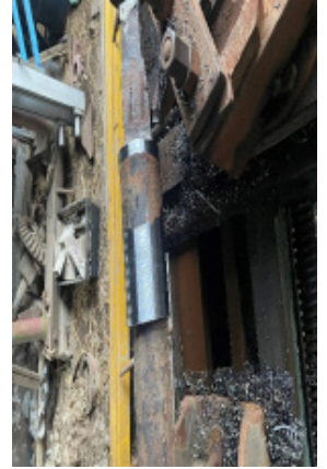
Machining of shaft to restore bearing surface
