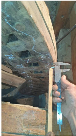
Checking the run-out.
